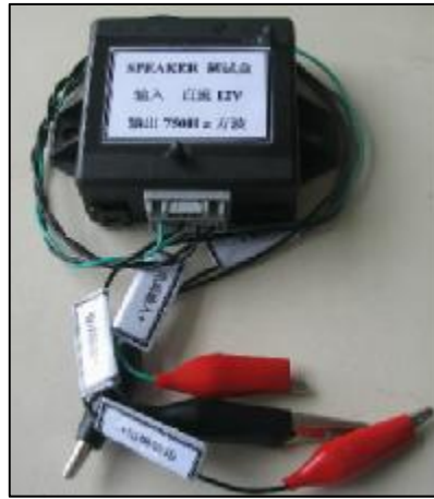
Fig 1: Customer SPL testing circuit:
