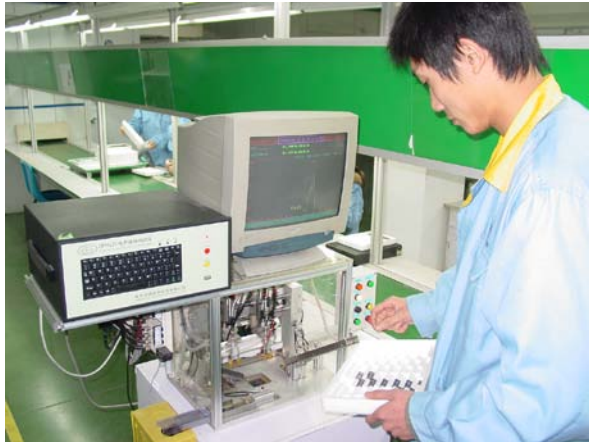
BeStar developed automated sound pressure level test module for surface mount components
