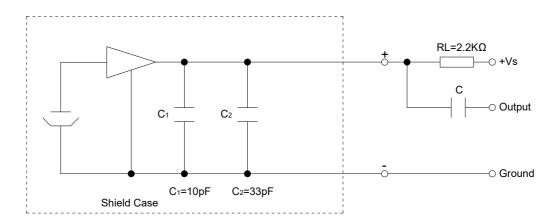
Figure 3. Schematic Diagram
