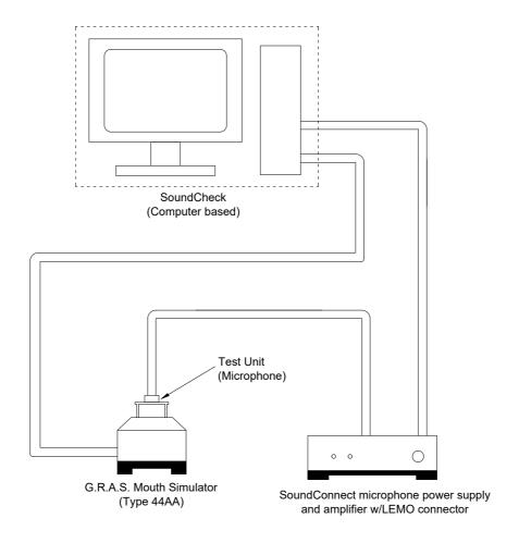
Figure 2. Test Setup
