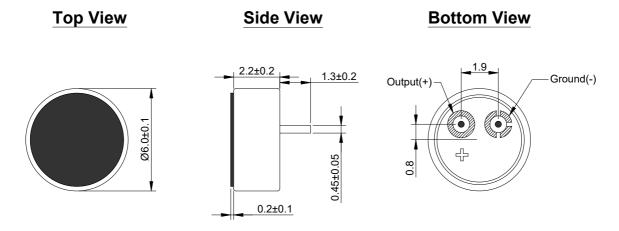
Figure 4. HBO0603B-52/1338 Mechanical Layout
