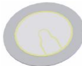
B1 – three-terminal circle with brim feedback, the metal is brass and Stainless Steel
